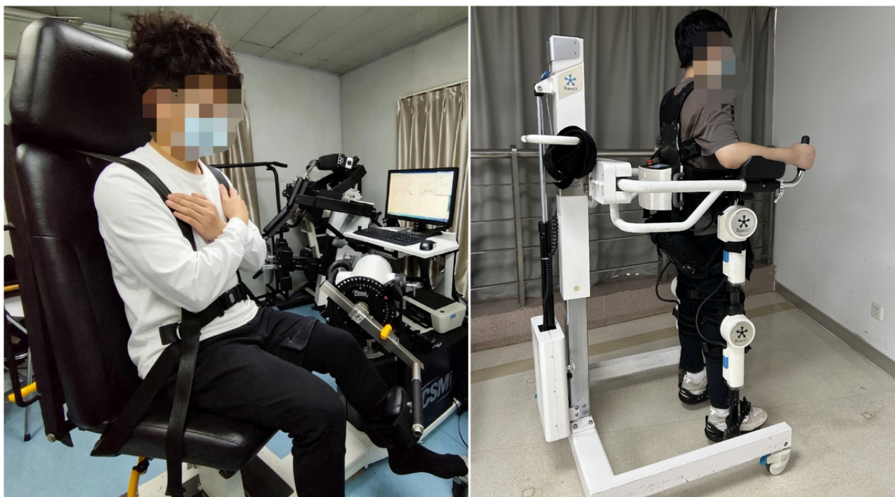
Figure 1. Isokinetic muscle strength testing of participants using the UGO rehabilitation exoskeleton (Chengtian) and Humac Norm isokinetic dynamometer (CSMi Solutions).
