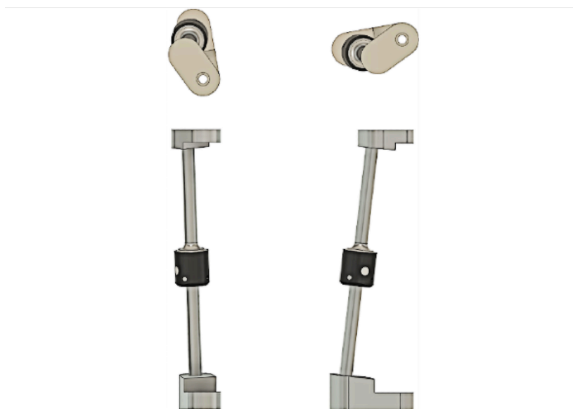
Figure 4. An example of a testing configuration for condition 2 of the test standard ISO (International Organization for Standardization) 10328: structural testing of lower limb prostheses (digital simulation render).
