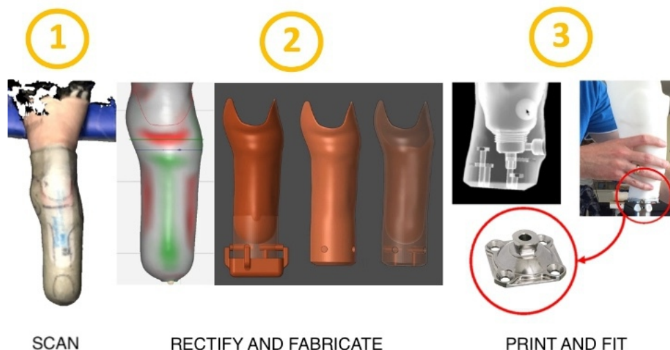
Figure 3. A typical digitalized process for 3D printing prosthetic sockets.
