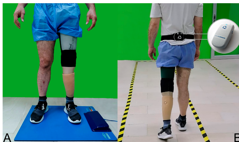
Figure 1. Experimental setup for gait assessment. (A) Plantar pressure recording during static standing; (B) Inertial sensor placement at the S1 level for dynamic gait analysis.
