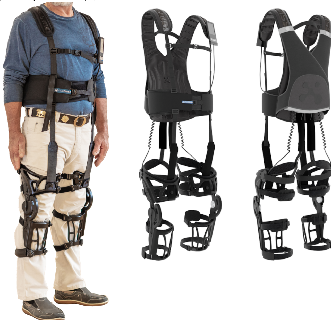
Figure 1. The Myosuit front and back perspective.
