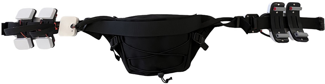
Figure 3. Picture of the new prototype of the haptic feedback device tested in this study.
