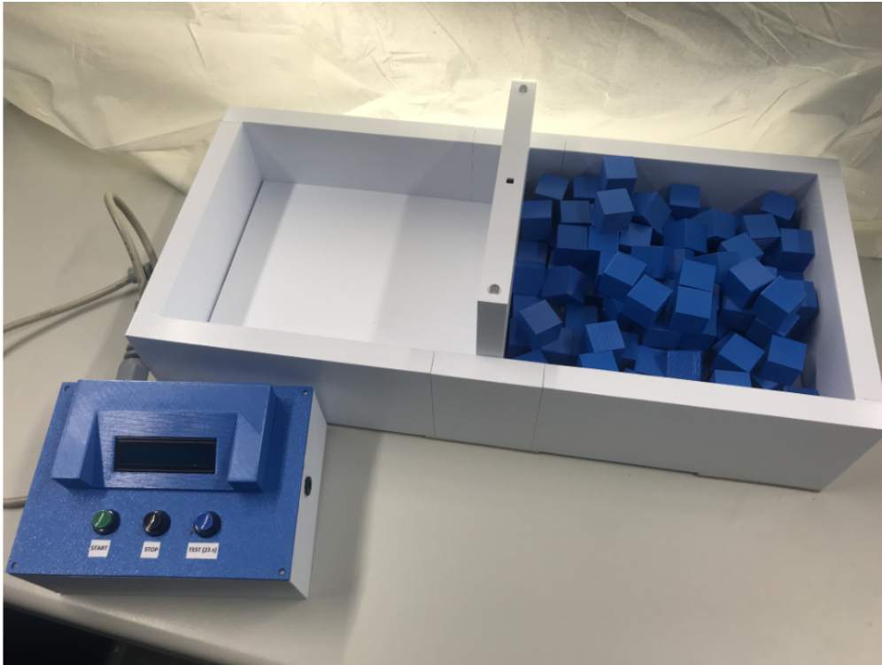
Figure 1. The components of the digital Box and Block Test board and control unit.
