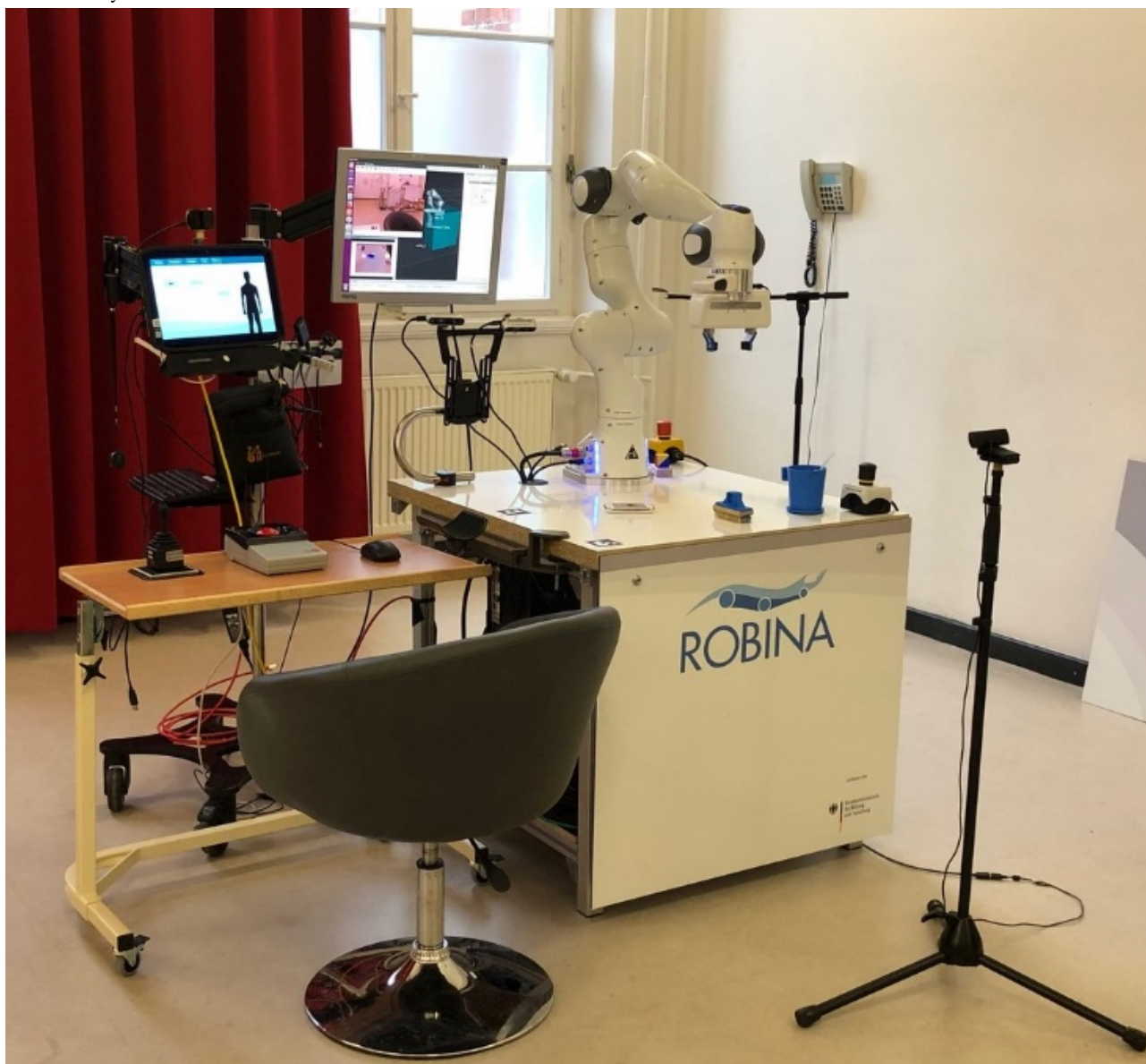
Figure 1. Evaluation setup of the robot-assisted services for individual and resource-oriented intensive and palliative care of people with amyotrophic lateral sclerosis system.
