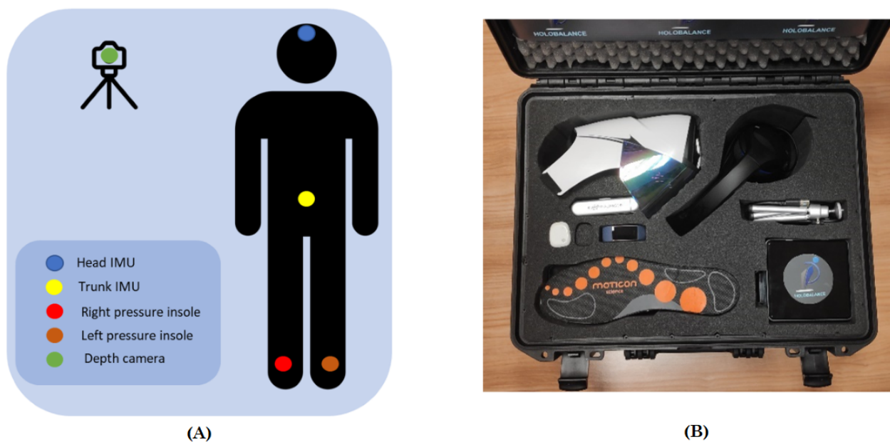
Figure 2. The Holobalance system. (A) Sensor positioning in the Holobalance system. (B) Devices of the Holobalance system. IMU: inertial measurement unit.
