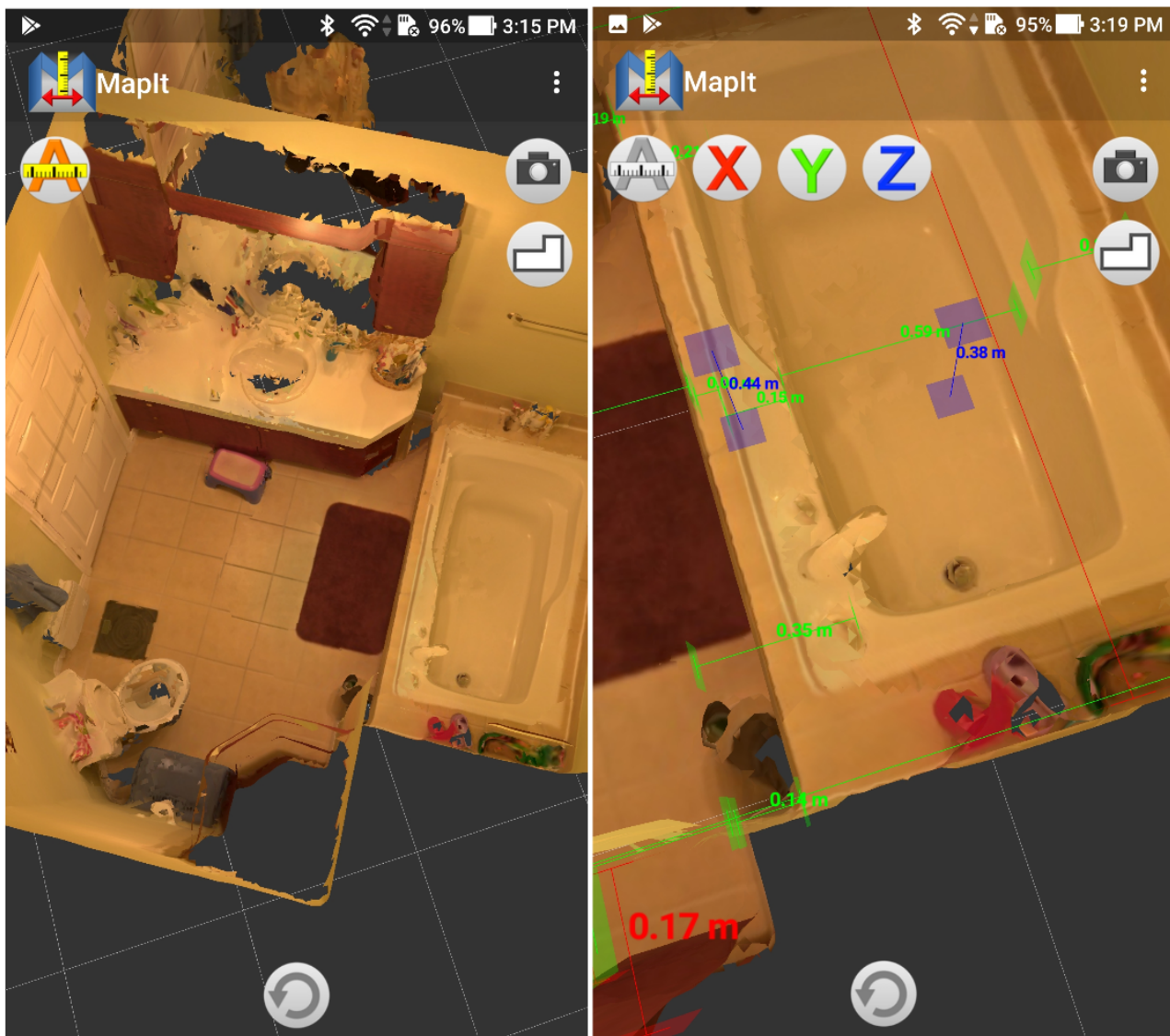
Figure 4. Phone app interface (V 0.4.1) when visualizing a scan. On the left, no automatic measurements were applied while on the right, automatic measurements are applied.
