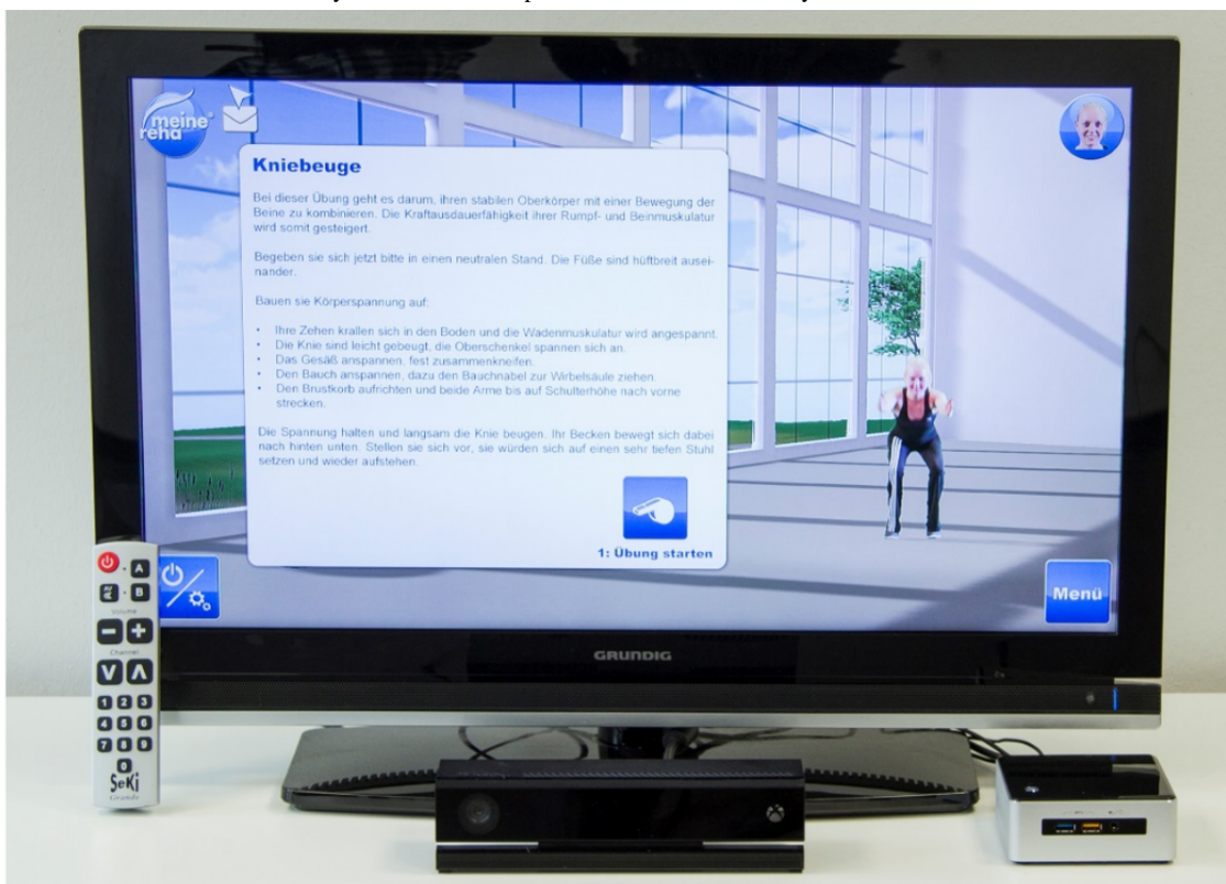
Figure 2. Hardware of the telerehabilitation system and an example exercise demonstrated by a virtual avatar.
