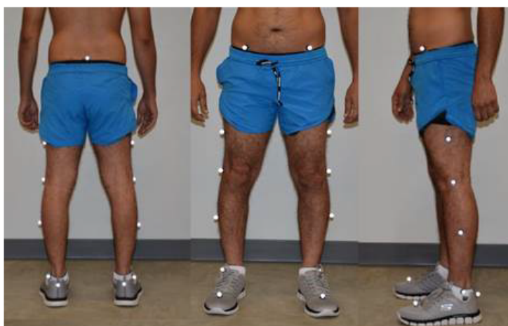
Figure 1. VICON Plug-In-Gait model lower extremity marker placements.
