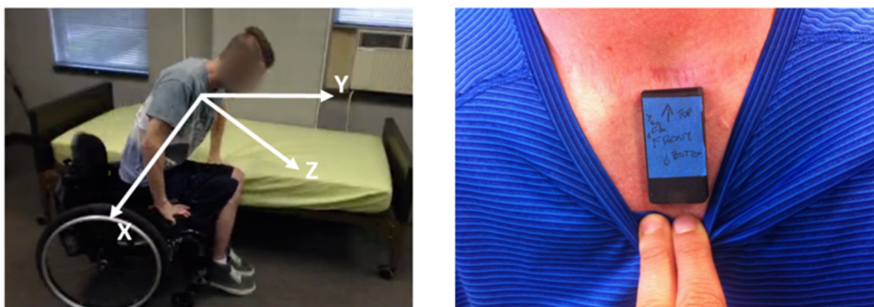
Figure 1. The orientation of the accelerometer's axes relative to the body during wheelchair transfers and its position on the participant's sternum.
