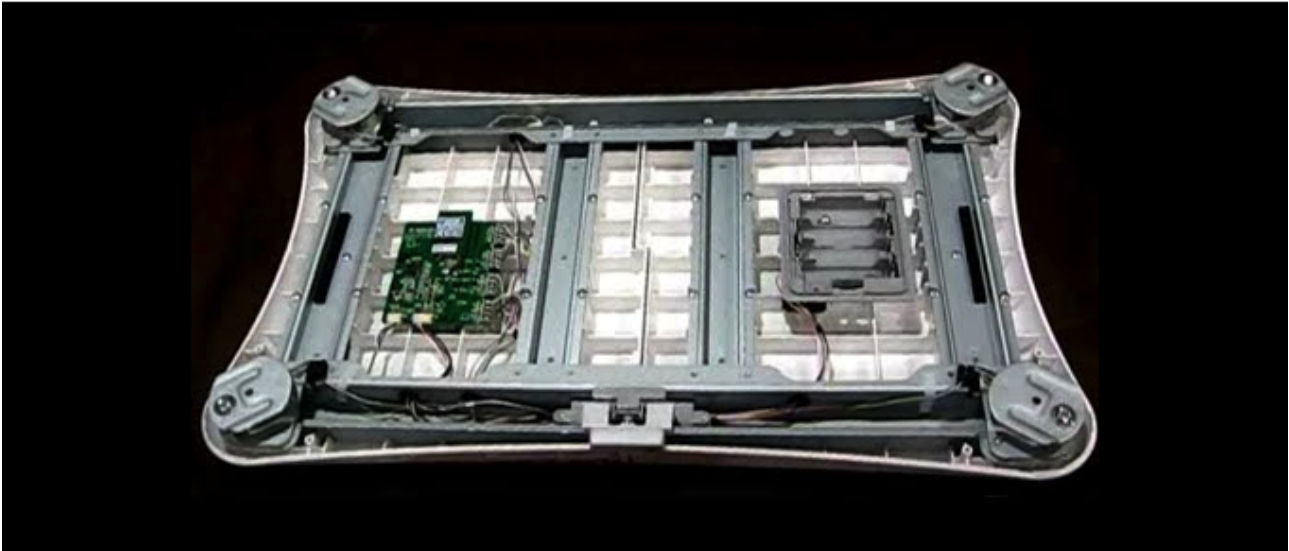
Figure 2. Wii Fit Balance Board electrical components.
