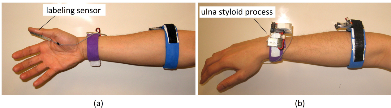
Figure 3. FSR straps placement: (a) forearm supinated view and (b) forearm pronated view.
